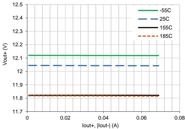
4.1.6 HTD1R5N-1212D Output Voltage vs. Current
