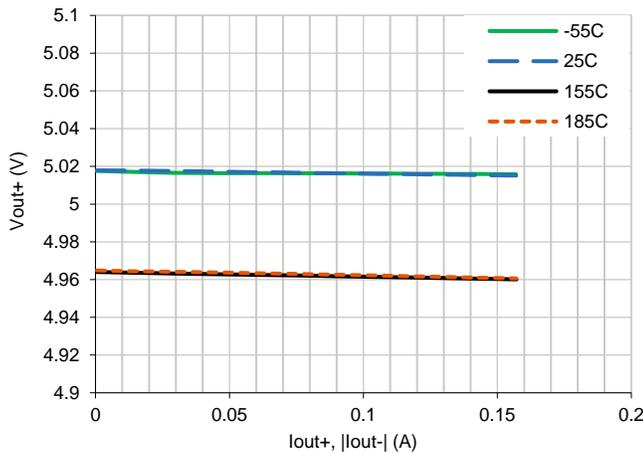
4.0.6 HTD1R5N-1205D Output Voltage vs. Current
